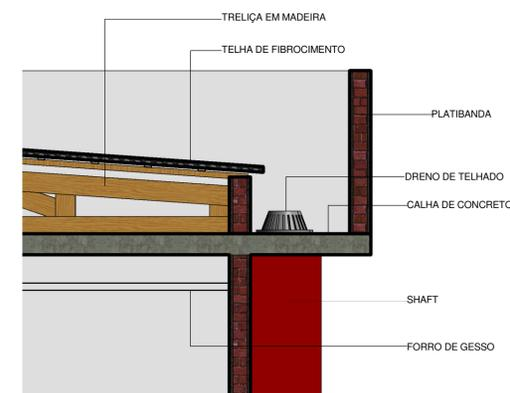
3 **CORTE DA PLATIBANDA**
